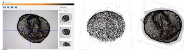
Fig. 4. On the left photography through a microscope (Micro-Capture Plus), in the middle a thick cloud in Agisoft Metashape showing the process of creating a 3D model, on the right an unedited 3D model of a coin with realistic texture and shape.
